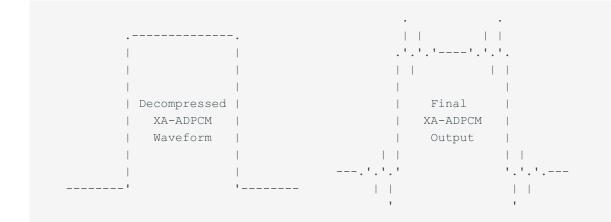
The zigzagging does produce some (inaudible) 22050Hz noise, and does produce some low-pass (?) filtering ("sinc filter"). The effect can be reproduced somewhat like so:
