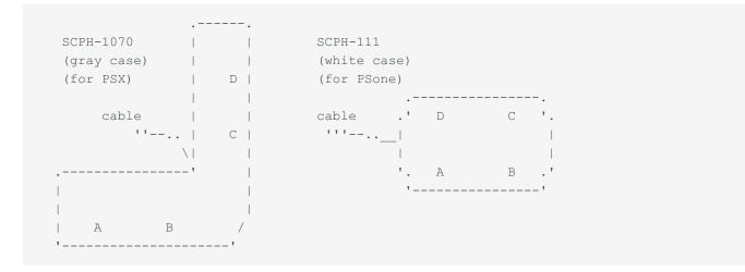
The cable connects to one of the PSX controller ports (which also carries the memory card signals). The PSX memory card port is left unused (and is blocked by a small edge on the Multitap's plug).
