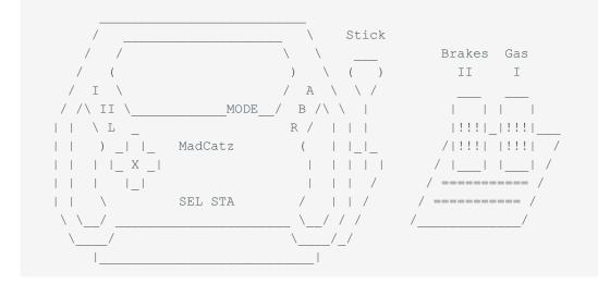
Unlike the neGon, the controller has Select, >\< and [] buttons, and a second set of L/R buttons (at the rear-side of the wheel) (no idea if L1/R1 or L2/R2 are at front?). Aside from the neGcon mode, the controller can be also switched to Digital mode (see below for button chart).
