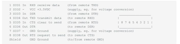
Can be used to communicate with another PSX via simple cable connection. With an external RS232 adaptor (for voltage conversion) it could be also used to communicate with a PC, a mouse, a modem, etc.
