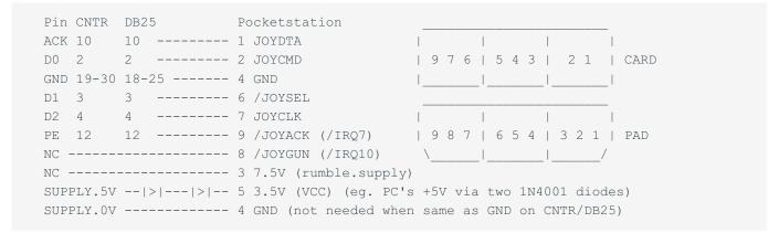
The circuit is same as for "Direct Pad Pro" (but using a memory card connector instead of joypad connector, and needing +5V from PC power supply instead of using parallel port D3..D7 as supply). Note: IRQ7 is optional (for faster/early timeout).
