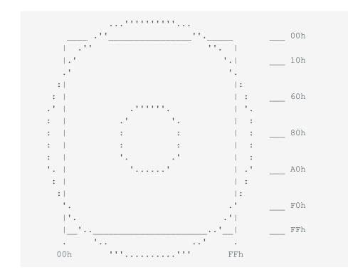
Big Circle--> Mechanically possible field of motionSquare Area--> Digitally visible 8bit field of motionSmall Circle--> Resting position when releasing the joystick
